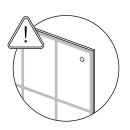
**Caution:** The French Silk Screen on our FSS Panels is a baked on, ceramic, matte black framing. This framing needs to be on the exterior of your shower enclosure once installed. The interior of the glass panel is coated with protective ENDURO SHIELD®, which will facilitate care and cleaning of your shower panel. This ENDURO SHIELD® coated side of your glass panel should face the interior/water side of your enclosure.
